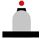
Projection of the laser dot at about 5 yards. The laser dot is just above the front sight when the sights are aligned properly.
